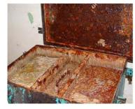
Figure 36: Severely corroded metal grease trap (these traps are highly prone to corrosion).
