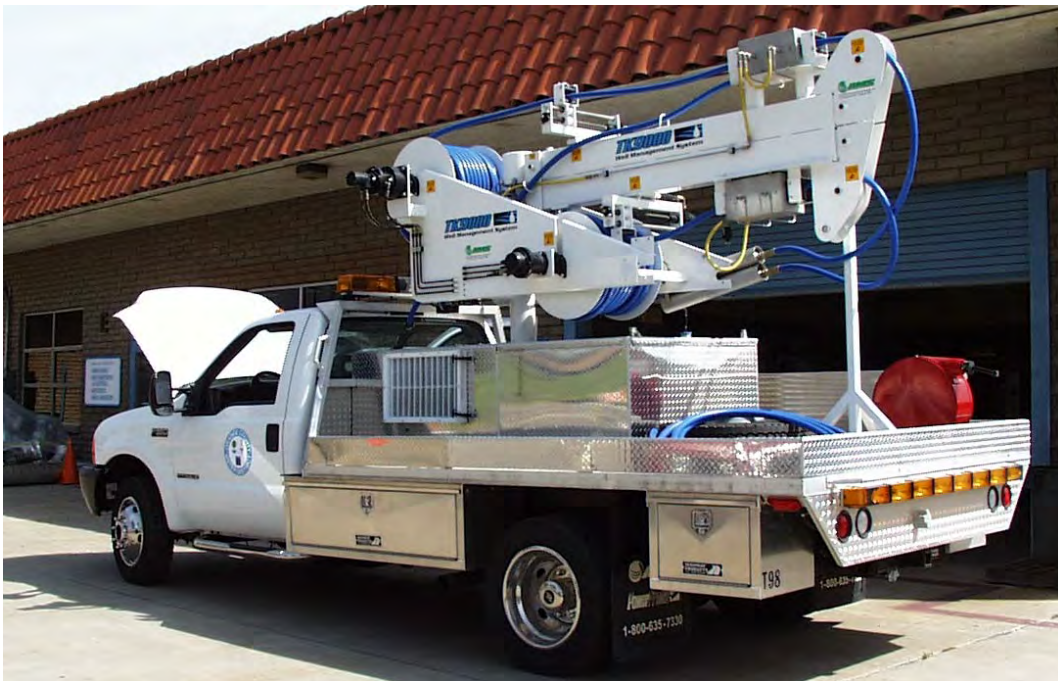
FIGURE 3-6 DUAL BOOM WATER QUALITY SAMPLING VEHICLE
